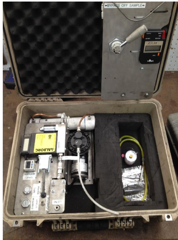
Figure 3.2 – Freudenberg portable sampling system
