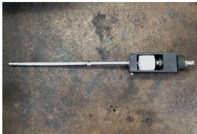
Figure 3.4 – ERP 21cm sampling probe for quartz filter collection
