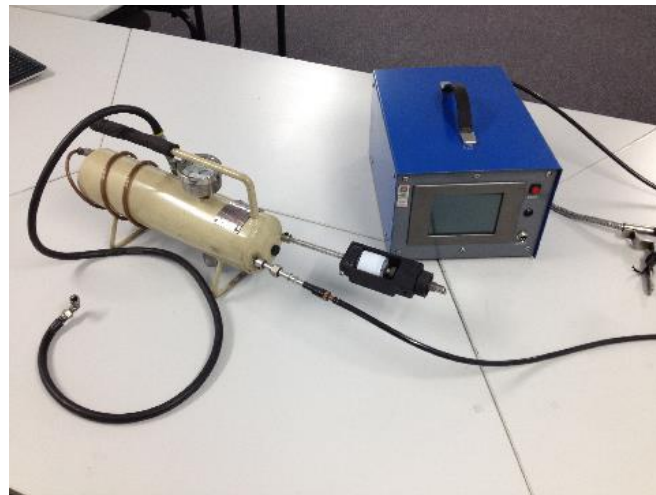
Figure 3.3 – ERP sampling chamber vessel with dual sampling probes
