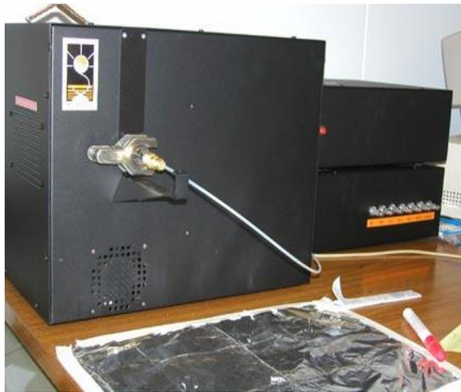
Figure 1 – The Sunset Industries Thermal/Optical Carbon Analyser
