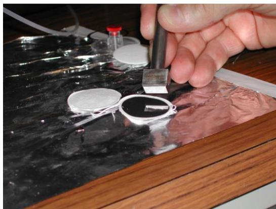
Figure 3 – 1.5cm<sup>2</sup> punch taken filter for analysis
