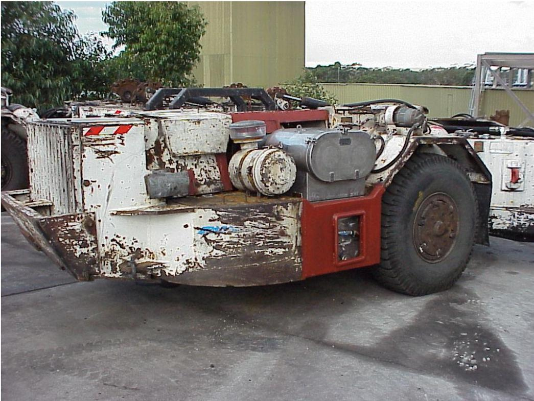
Figure 16 – Disposable filter assembly fitted to an underground mining machine (Source: B Davies)
