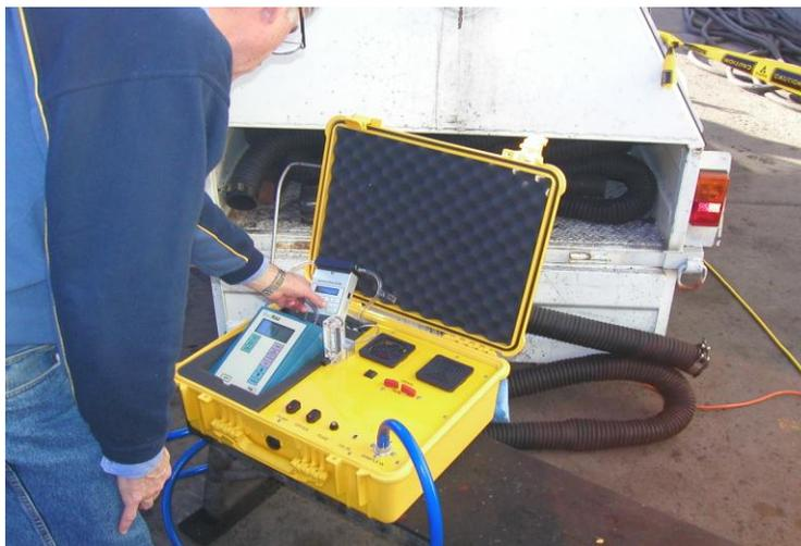
Figure 15 – Air Quality Industries DPM in Exhaust Measurement Instrument
