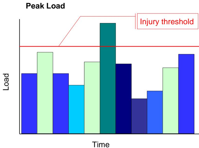
**Figure 3-1** *Injury caused by peak loading*
