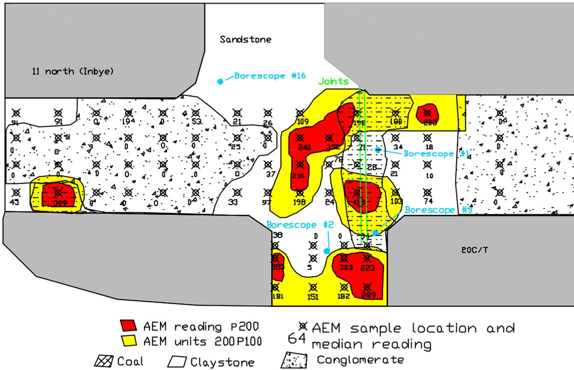
Figure 5.5 Claystone/sandstone roof lithology with geological structure
