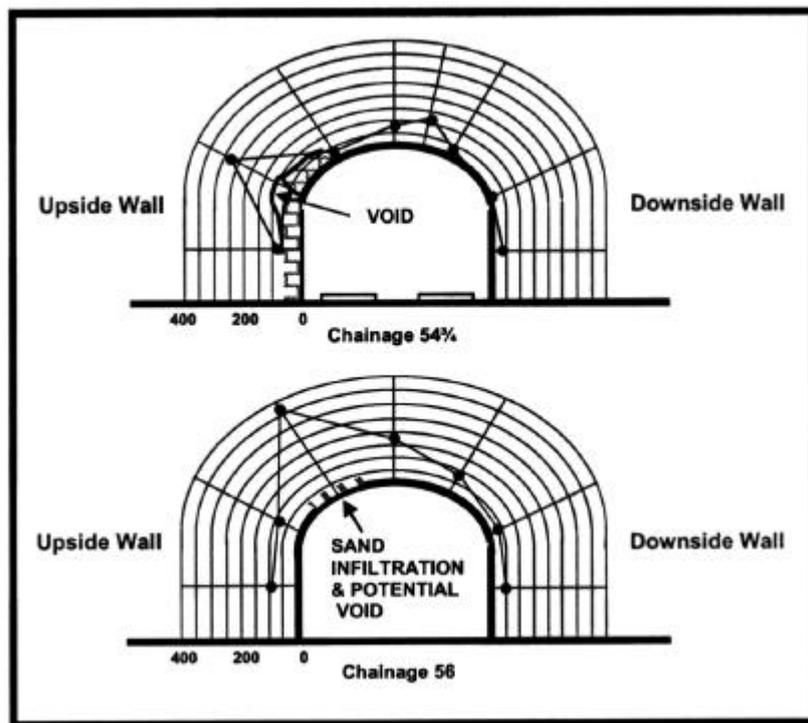
**Figure 2.7. AEM Survey Results – Brick Lined Tunnel**
