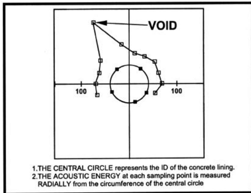
**Figure 2.8. AEM Survey Result – Concrete Segmental Lining**
