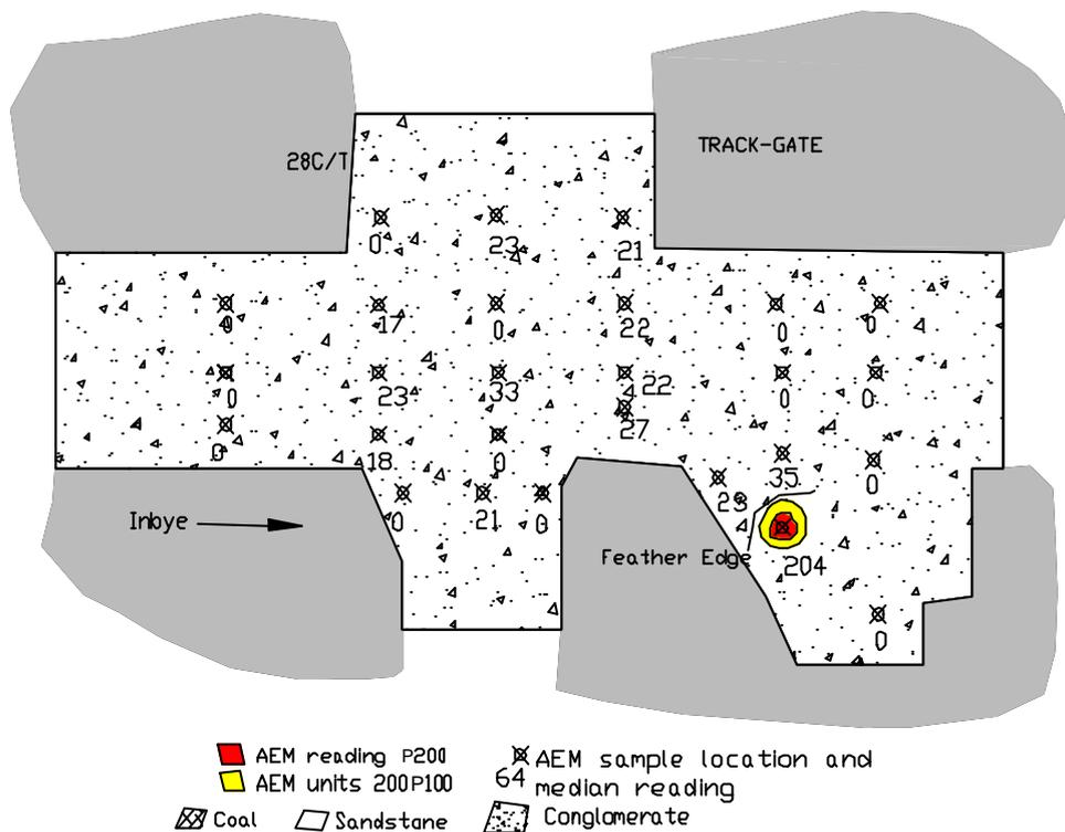
**Figure 5.2 Conglomerate roof test area with feather edge/fracture.**
