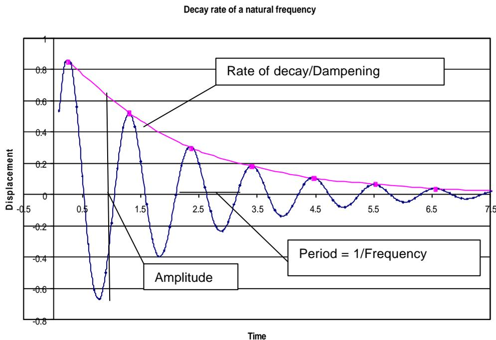
**Figure 2.1 Decreasing amplitude, frequency and the rate of decay for a vibration. Based on relationships from Meriam & Kraige (1993).**
