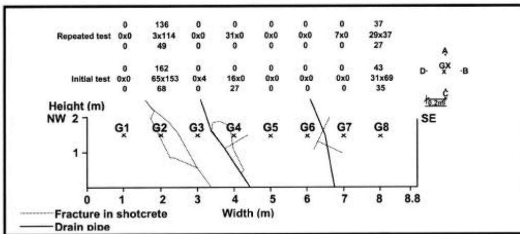
**Figure 2.9. Test Configuration and Results from the AEM Test Profile in a Pillar with a Shotcrete Lining**
