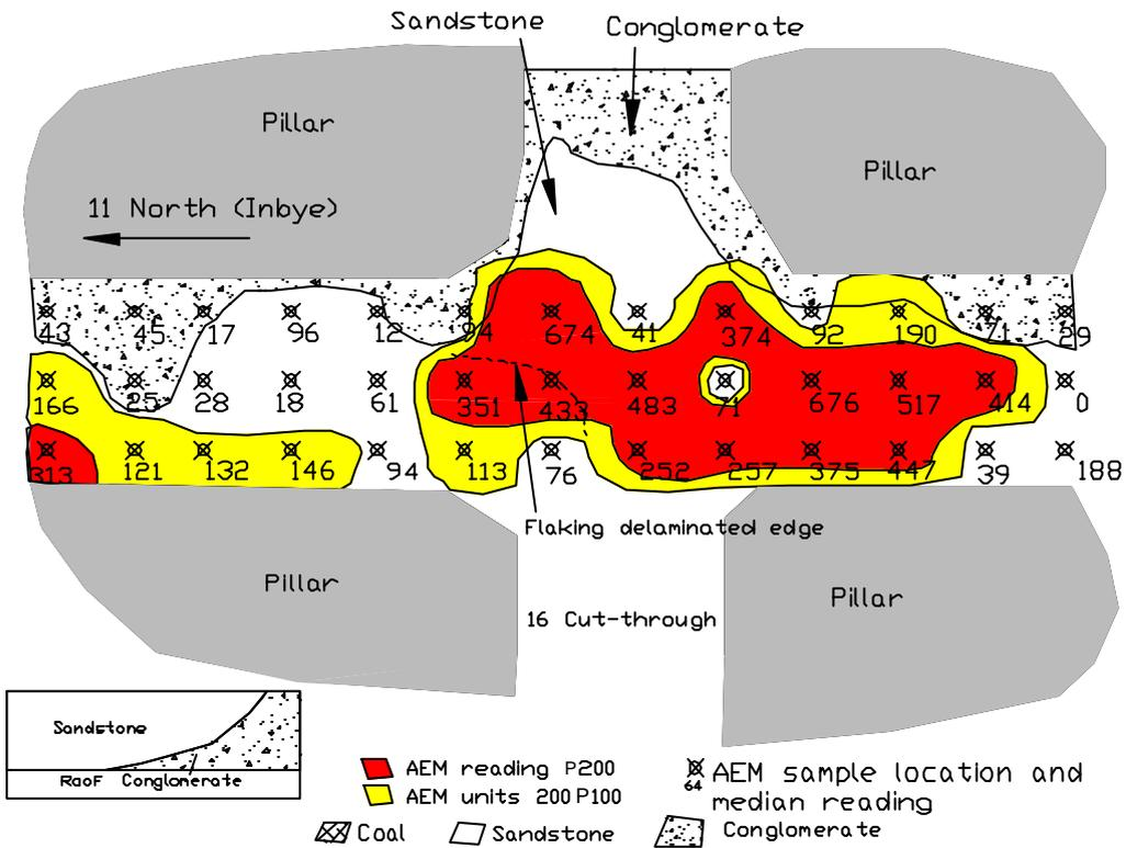
Figure 5.6 Sandstone roof lithology with geological structure
