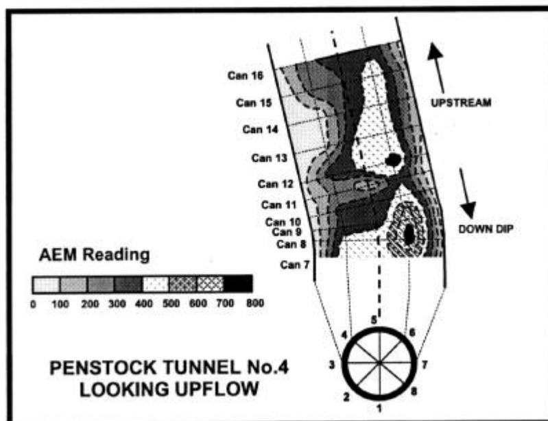
**Figure 2.6. Relief Plot in Plan View Showing Contours of AEM Readings**
