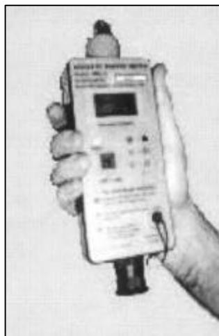
**Figure 2.2. RDL4 Acoustic Energy Meter**
