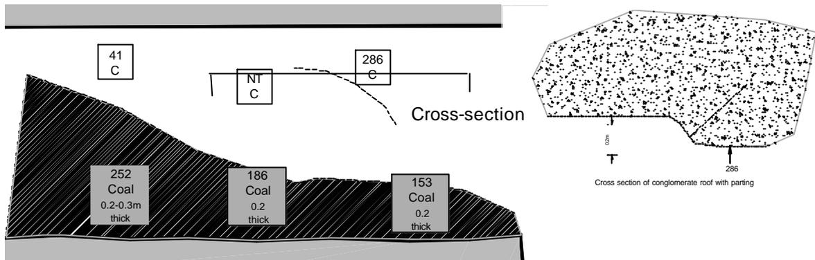
**Figure 5.7 Conglomerate roof with open geological structure**
