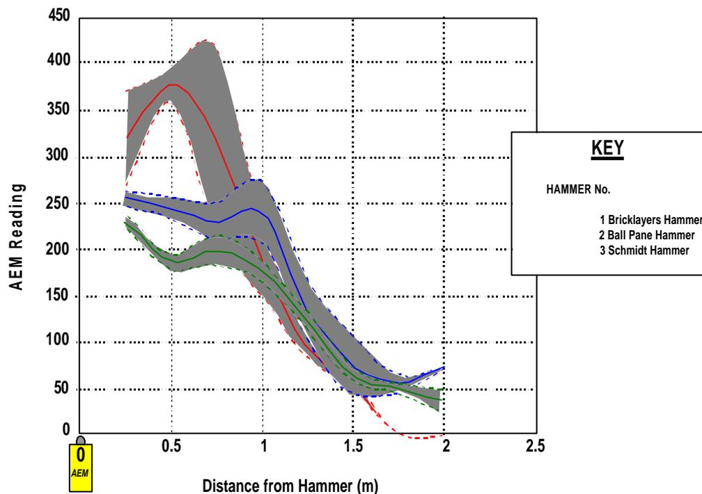
**Figure 2.4. Plots of AEM Reading with Respect to Hammer Type and Hammer Impact Point**
