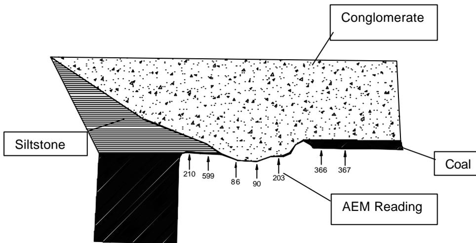
**Figure 3.1 Lithological contacts with an AEM traverse.**
