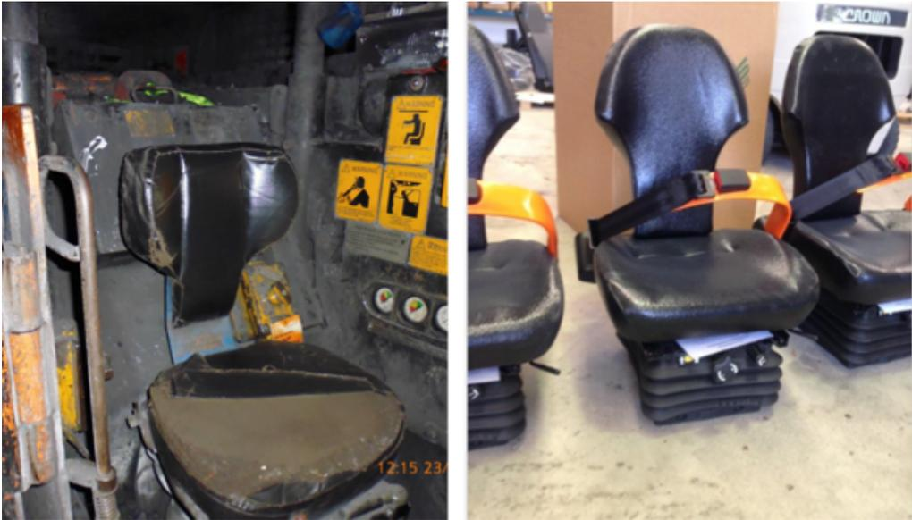
Figure 9: Seat condition before replacement and new seats awaiting installation.
