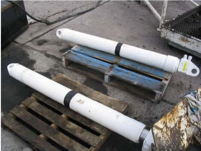
Figure 1: The DA-Rams have had a line painted on them to indicate the best strapping point.
