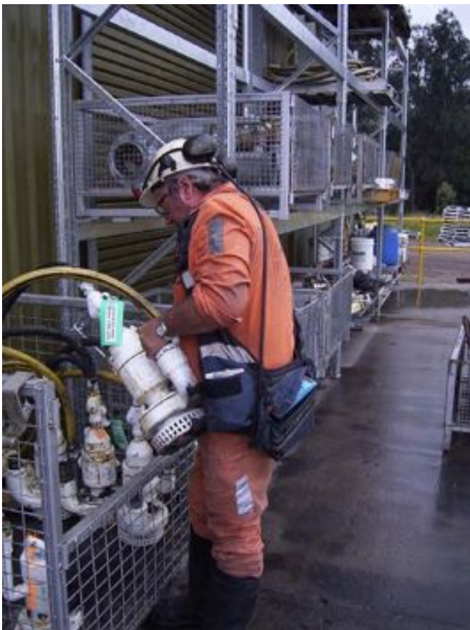
Figure 3: Lifting a 'screamer' pump out of a 'low' storage bin.
