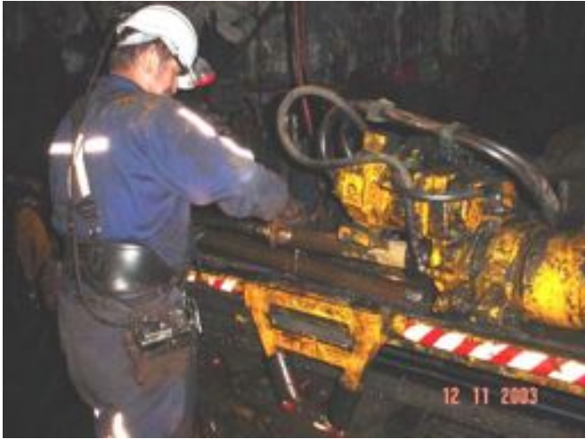
Figure 1: Removing water swivel on gas drainage tube
