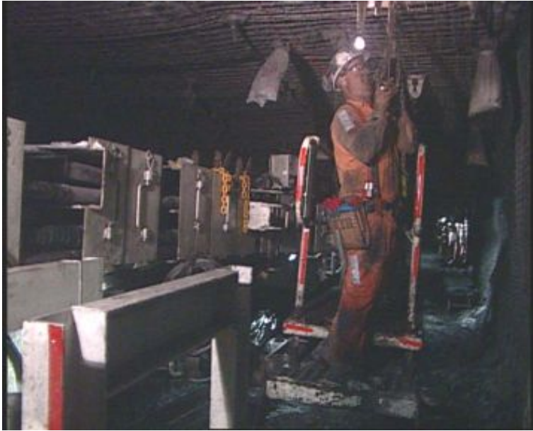
Figure 1: Removing a monorail section from the platform attached to the main gate.
