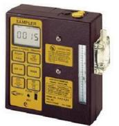
Figure 7 – SKC Air Sampling Pump
