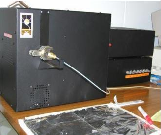
Figure 1 – The Sunset Industries Thermal/Optical Carbon Analyser
