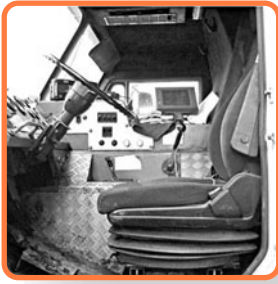
The driver's space may be insufficient to allow full adjustment of the seat.
