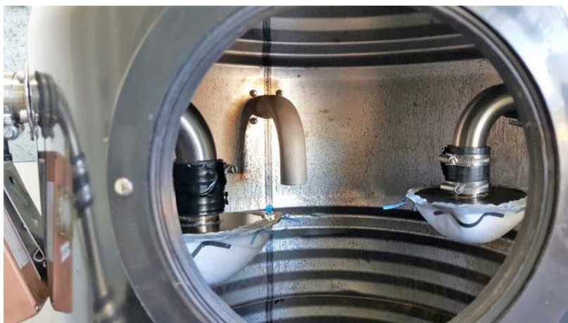
Figure 3-34: Filter Samples Mounted Inside the Experimental Chamber Showing Post Filter Port A, Post Filter Port B and the Pre Filter Sampling Port.
