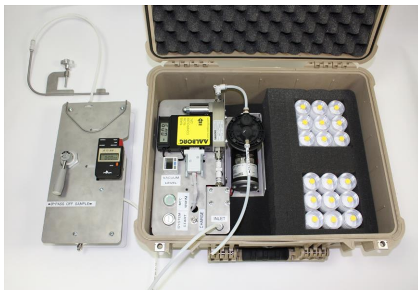
Figure 6.4 - Freudenberg sample collection system
