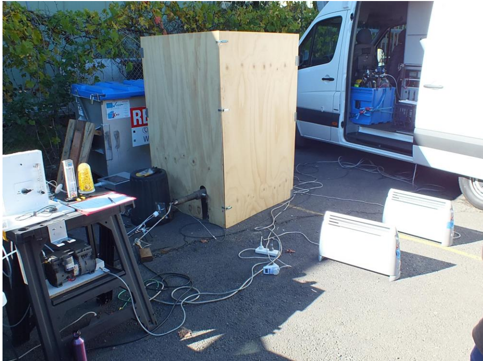
Figure 4.6 – Noise barrier around DP generator
