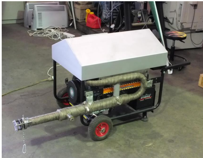
Figure 4.4 - DP generator with exhaust mixing system
