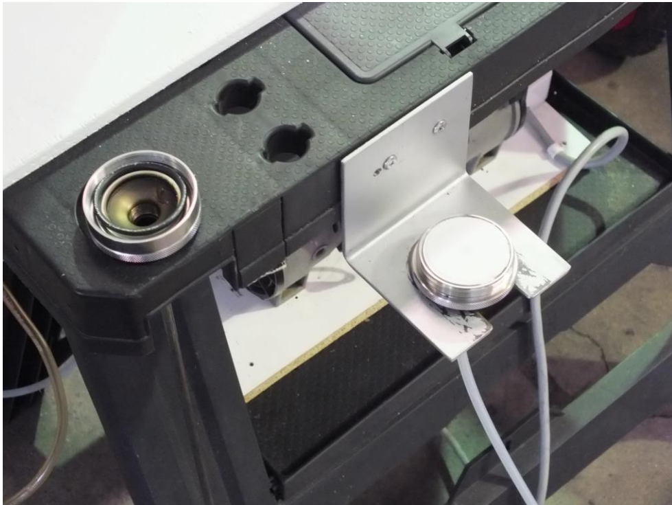
Figure 4.8 – Sample probe and filter holder assembly
