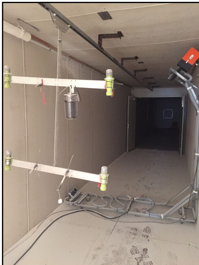
Figure 4.4.1: Test rig with blast protection enclosure on picture left and 'Dust Hunter' picture right side.
