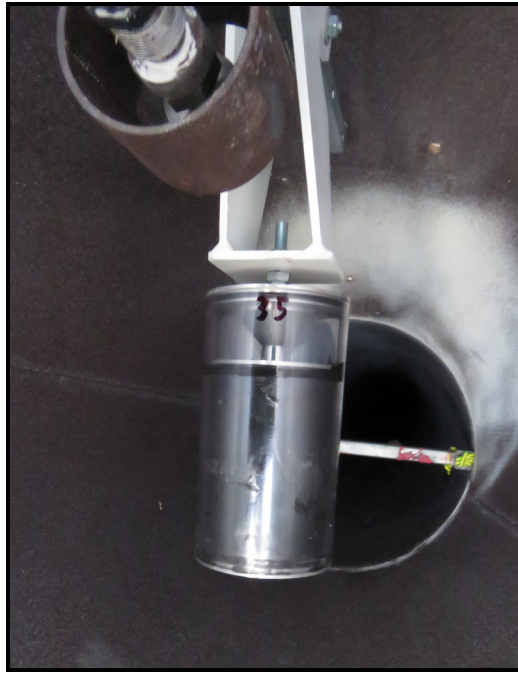
Figure 5.3.3: Prototype polycarbonate enclosure.
