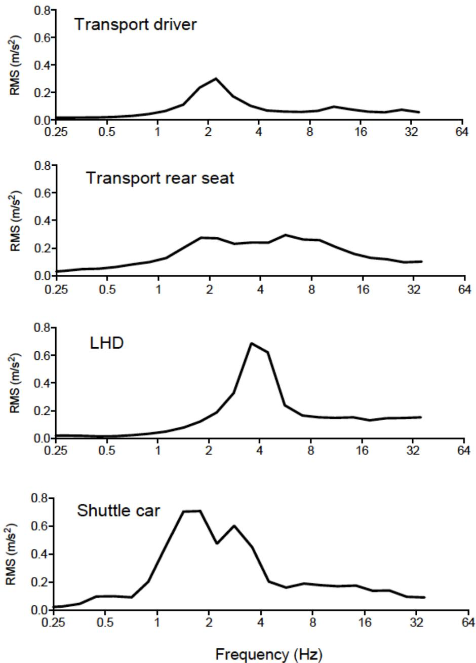
Figure 3: Frequency spectra for vertical whole-body acceleration measurements taken from a range of underground coal mining equipment.
