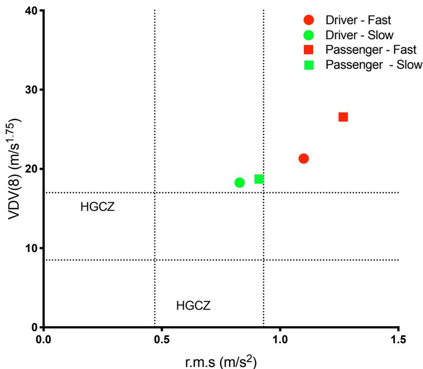
Figure 11: Vertical whole-body vibration amplitude for SMV driver and front passenger at slow and fast vehicle speeds.
