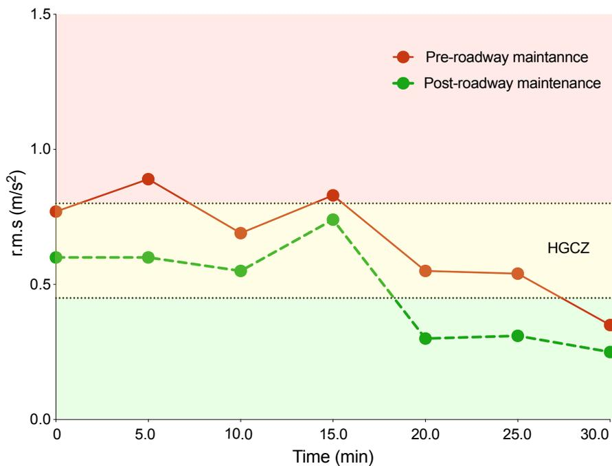
Figure 14: Vertical whole-body vibration amplitude for SMV driver at 5 minute intervals for the same section of roadway before and after maintenance.
