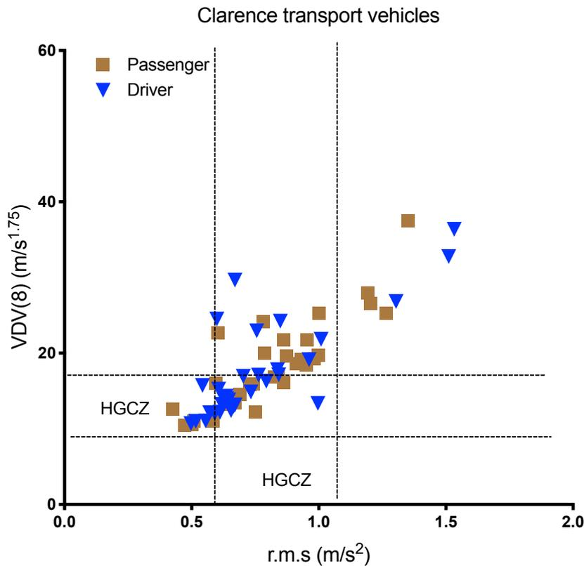
Figure 6: Vertical whole-body vibration measurements taken from personnel transport vehicles (SMV/PJB) at Clarence underground coal mine. The data are provided for driver and passenger and expressed as VDV(8) and r.m.s. with respect to the ISO2631.1 Health Guidance Caution Zone (HGCZ) for an 8 hour daily exposure.
