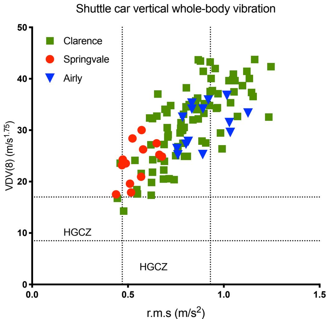
Figure 4: Vertical whole-body vibration measurements taken from shuttle cars at three underground coal mines. The data are expressed as VDV(8) and r.m.s. with respect to the ISO2631.1 Health Guidance Caution Zone (HGCZ) for an 8 hour daily exposure.
