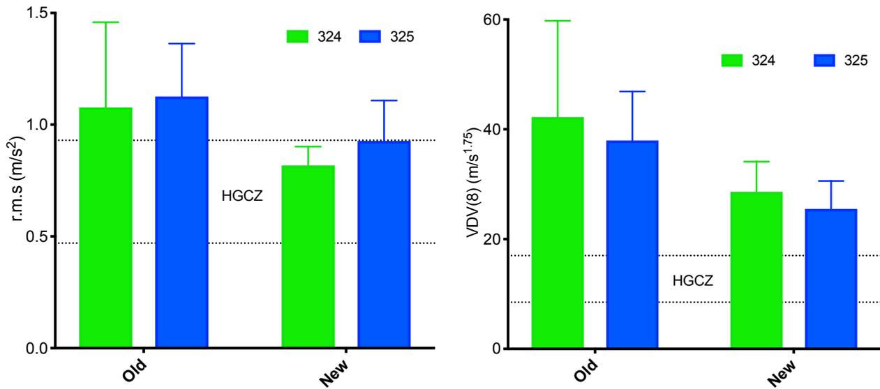
Figure 10: r.m.s. (left panel) and VDV(8) (right panel) vertical whole-body vibration measurements from two shuttle cars before and after seat replacement (mean and SD).
