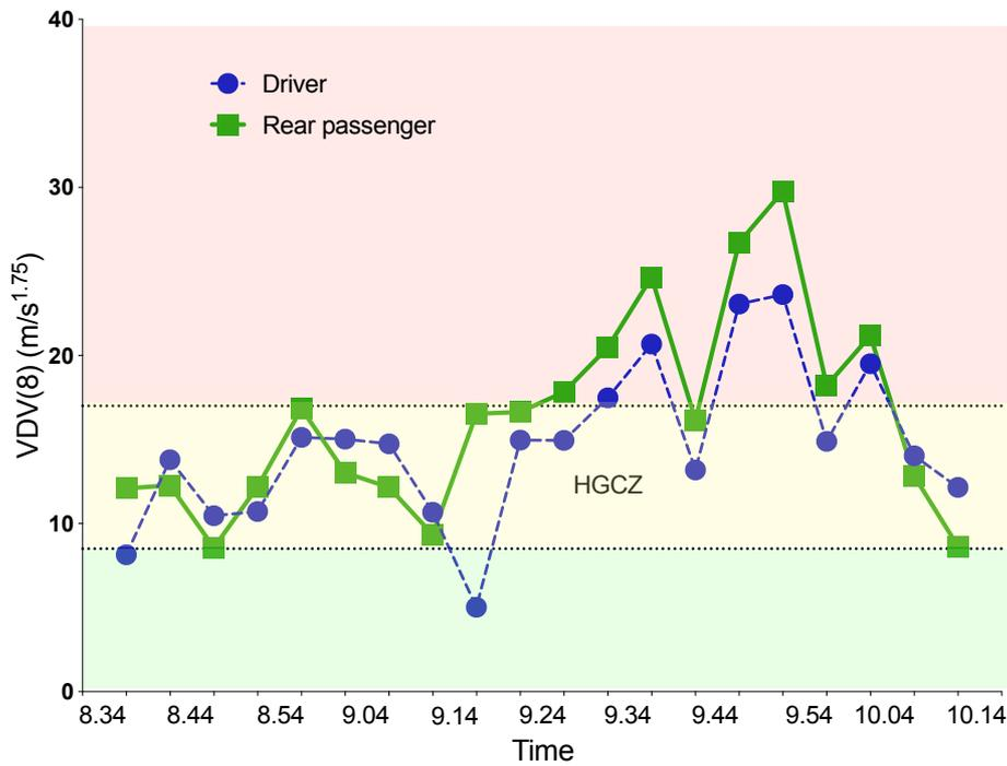
Figure 13: Vertical whole-body vibration amplitude for SMV driver and front passenger at 5 minute intervals during for driver and rear passenger while navigating the main travel road.
