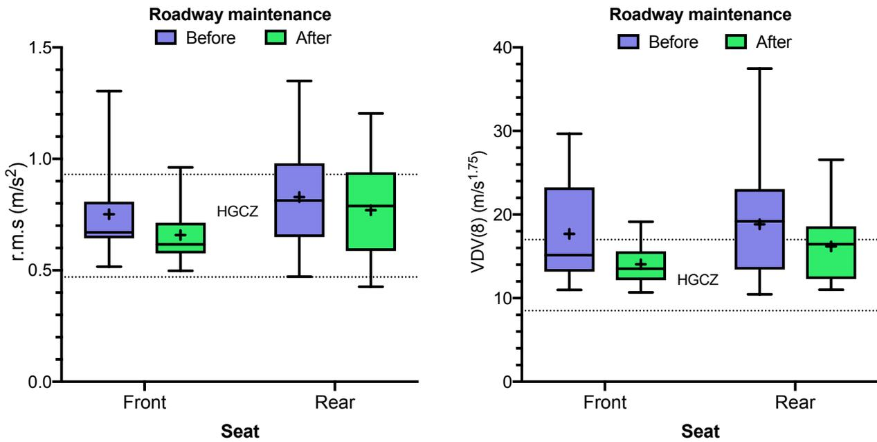
Figure 15: Vertical whole-body vibration amplitude for SMV driver at 5 minute intervals for the same section of roadway before and after maintenance.
