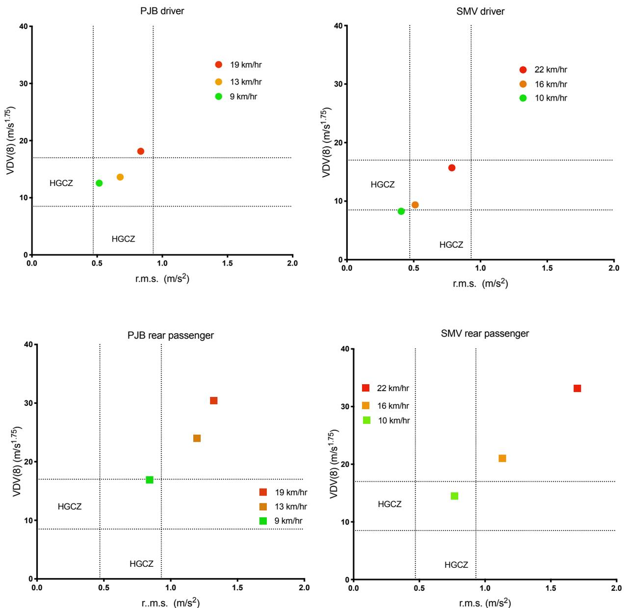
Figure 12: Vertical whole-body vibration amplitude for SMV and PJB driver and rear passenger at slow and fast transport vehicle speeds.
