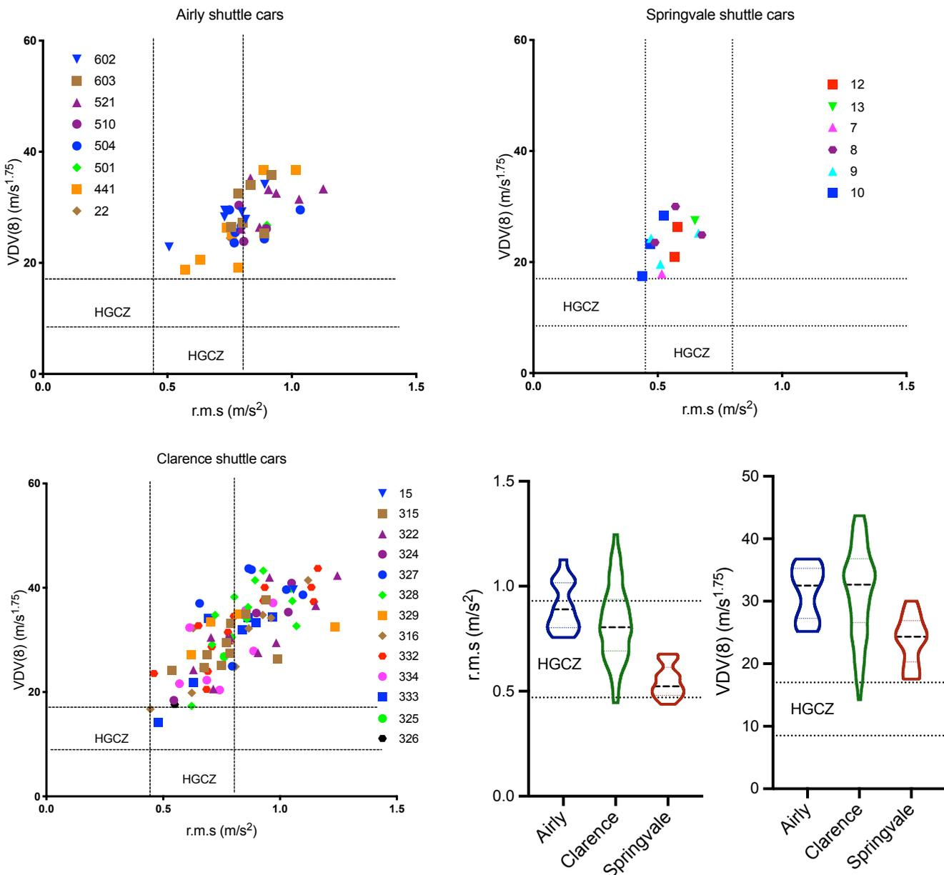
Figure 5: Vertical whole-body vibration measurements taken from shuttle cars at three underground coal mines for individual shuttle cars. The data are expressed as VDV(8) and r.m.s. with respect to the ISO2631.1 Health Guidance Caution Zone (HGCZ) for an 8 hour daily exposure.
