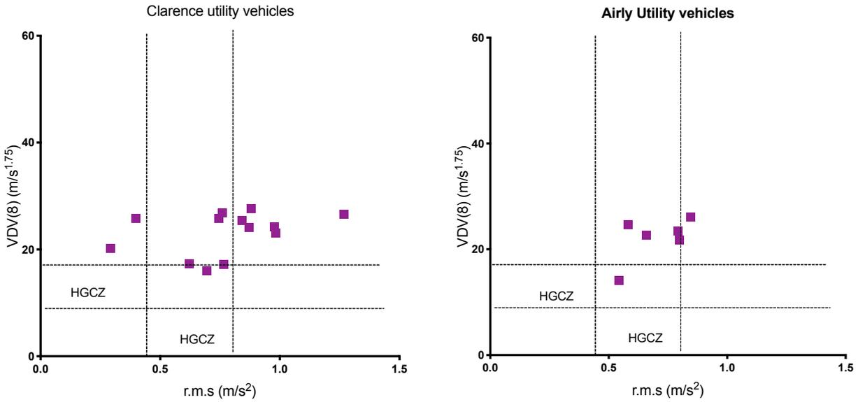
Figure 7: Vertical whole-body vibration measurements taken from utility vehicles (LHD's) at Clarence and Airly mines. The data are expressed as VDV(8) and r.m.s. with respect to the ISO2631.1 Health Guidance Caution Zone (HGCZ) for an 8 hour daily exposure.
