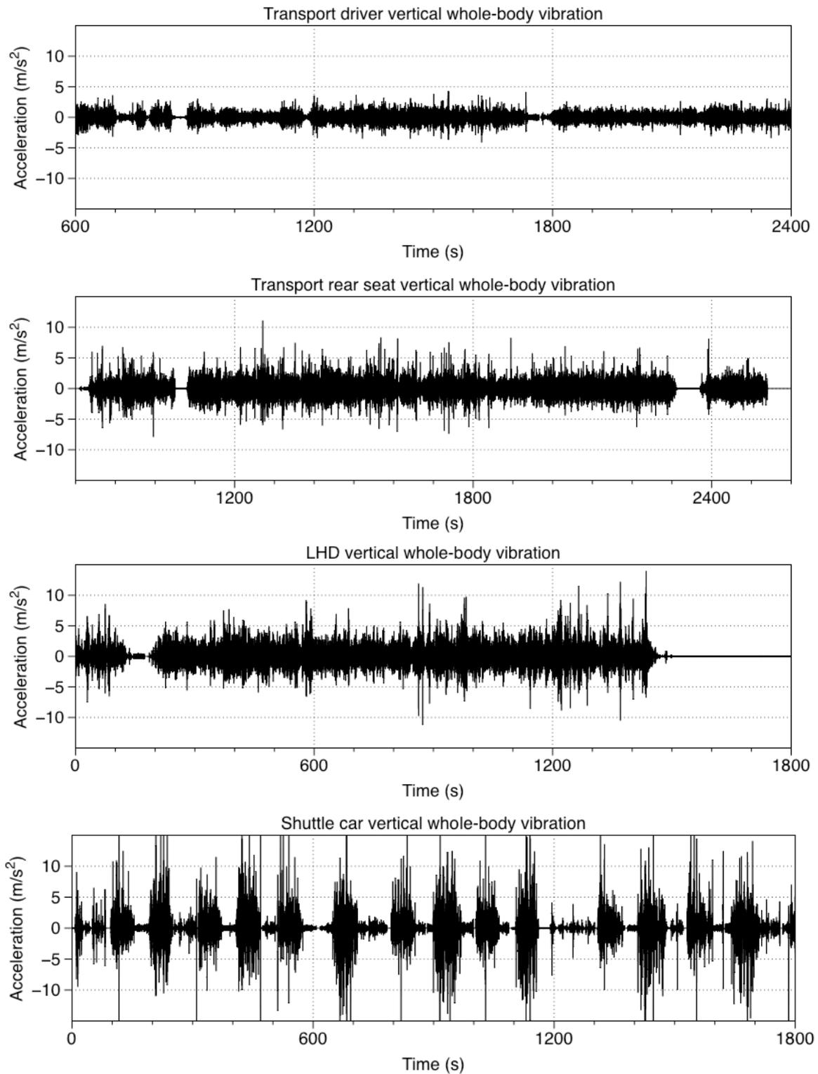
Figure 2: Frequency weighted vertical whole-body vibration samples taken from a range of underground coal mining equipment.
