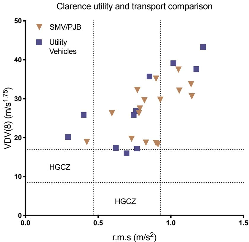
Figure 8: Comparison vertical whole-body vibration measurements taken from personnel and supply vehicles at Clarence mine. The data are expressed as VDV(8) and r.m.s. with respect to ISO2632.1 Health Guidance Caution Zone (HGCZ) for an 8hour daily exposure.
