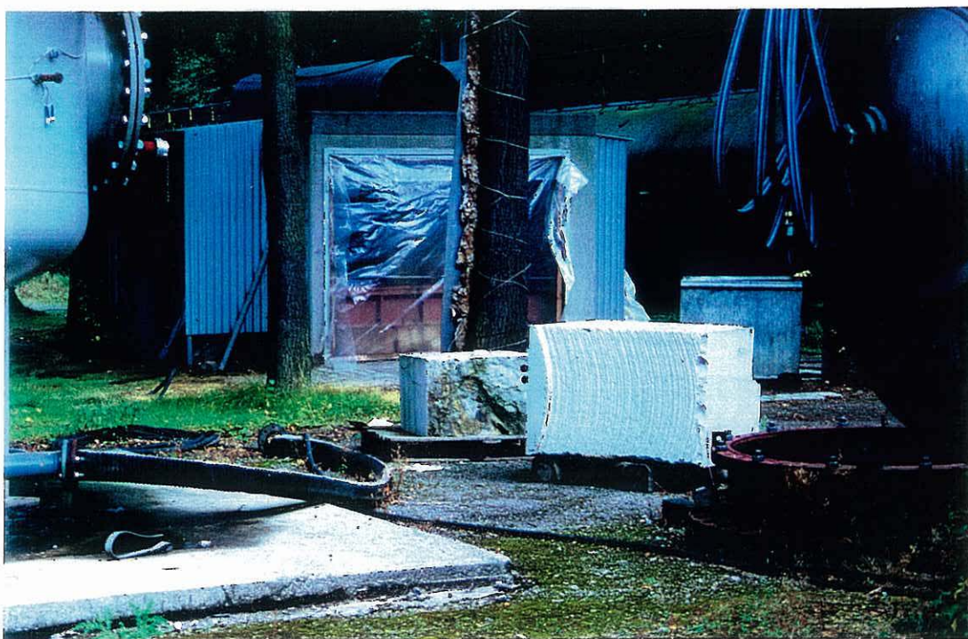
Figure 7.3: General view of frictional ignition test facility at DMT Gesellschaft für Forschung und Prüfung, Dortmund, Germany, showing plastic blow-out wall in place. A rock sample block, after cutting in the chamber, can be seen in the foreground.
