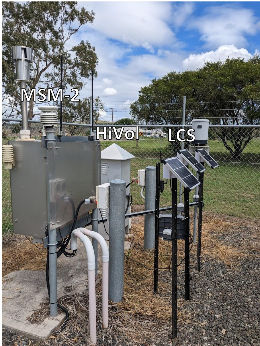
Figure 16: Mine site monitoring station – six LCS next to HiVol (reference) and MSM-2 (near-reference) methods.
