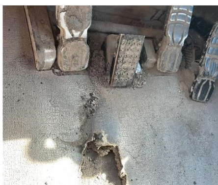
Above: Example of poor cabin floor conditions that contributed to a worker exceedance of the RCS workplace exposure standard.
