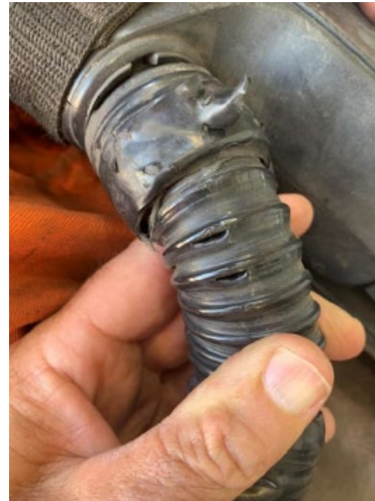
Poorly maintained PAPER units
